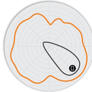
Figure 5. R650 5GHz Elevation Antenna Patterns
